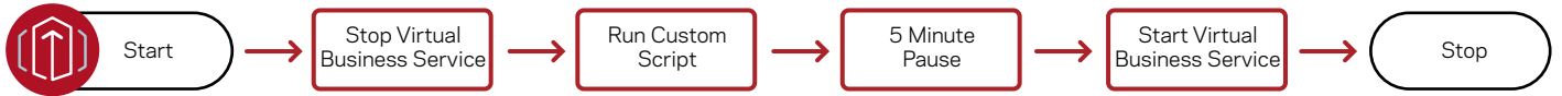
Figure 8. An example of the resiliency plan for automated failover of an IT business service.
